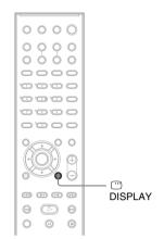
Use the Control Menu to select a function and to view related information. Press DISPLAY repeatedly to turn on or change the Control Menu display as follows:
